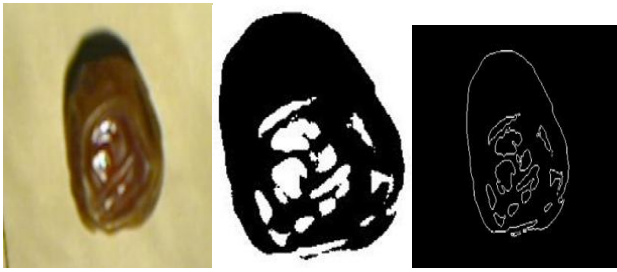
Figure-3: Figure shows an original date image, its binarised image and edges which surrounds this binarised image. [12]
