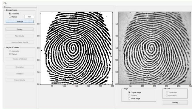
Fig. 15: original fingerprint and its binarization image.
