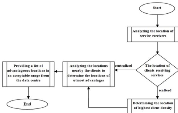
Figure. 6 the sub-procedure of locating candidate places
