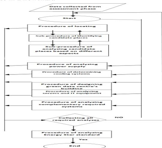
Figure. 3 different stages of implementing analysis phase
