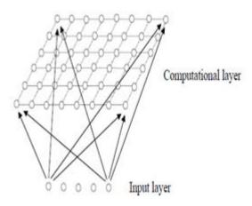
Figure 3. Feed-forward structure of Kohenon SOM network
