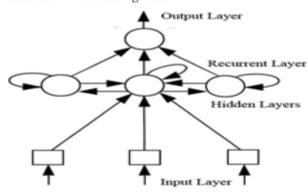
Figure 2. Structure of Layer Recurrent Neural Network
