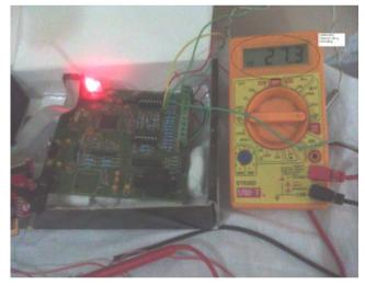
Figure. 5. Current Measurement in Transmitting Mode
