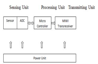
Figure.2. Block Diagram of Slave Mote
