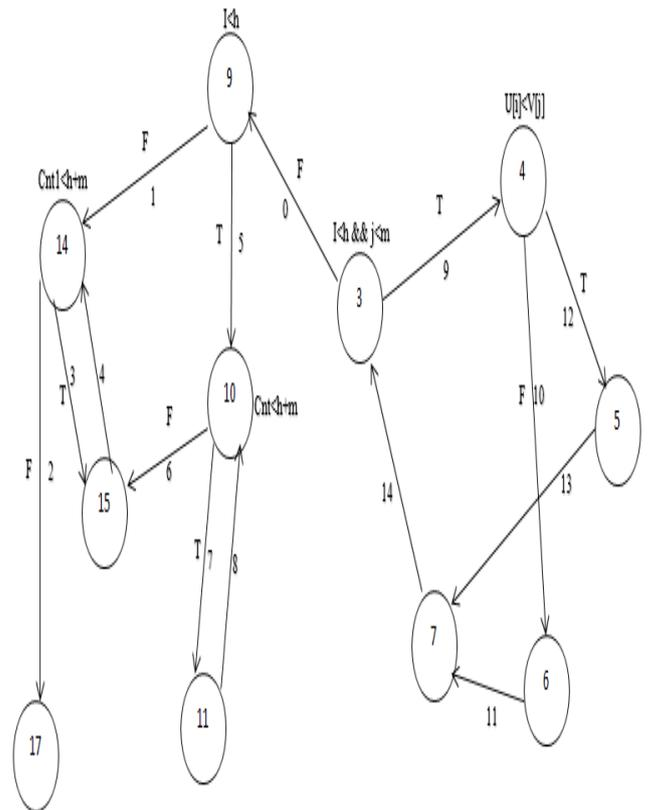
Figure 2. Program flow graphs merging two sorted arrays.
