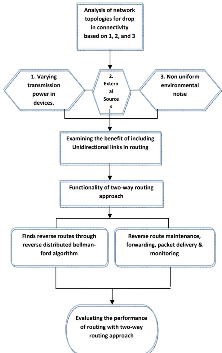
Figure 1. Handling unidirectional links in AODV
