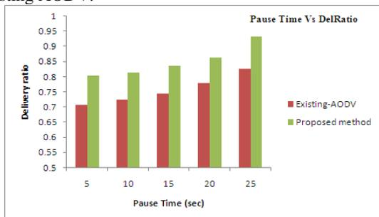
Figure 4. Pause Time Vs Packet Delivery Ratio
