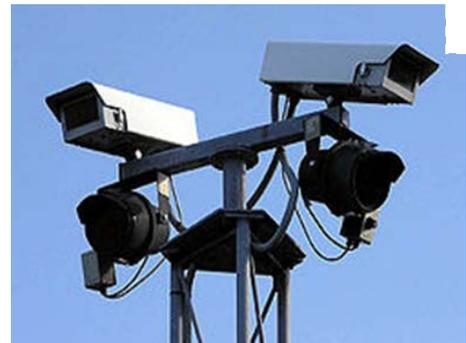
Figure. 6. Camera Used In ANPR Technology
