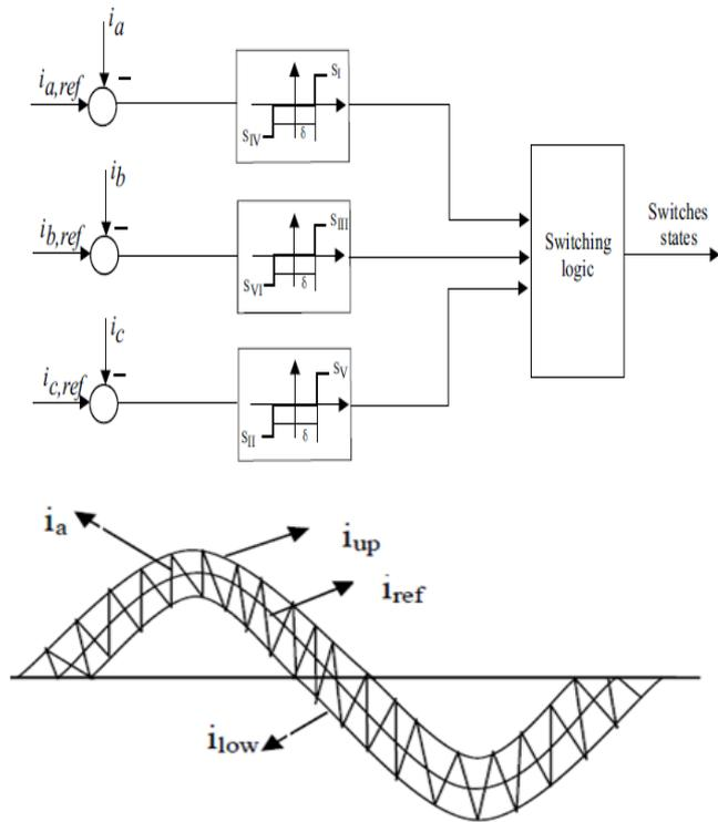
Figure 5 (a) Basic circuit diagram of hysteresis controller (b) hysteresis controller control structure
