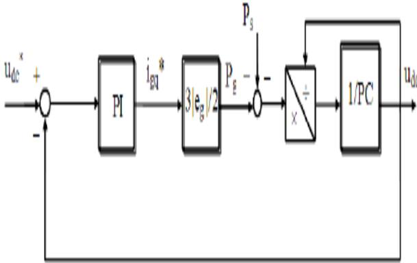
Figure: 4 Block diagram of closed loop control of DC Link voltage
