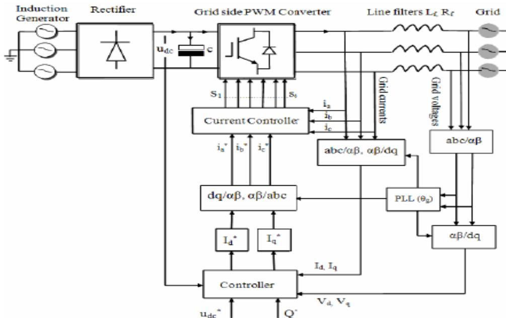
Figure 3 Block diagram of virtual grid flux control of grid connected VSI
