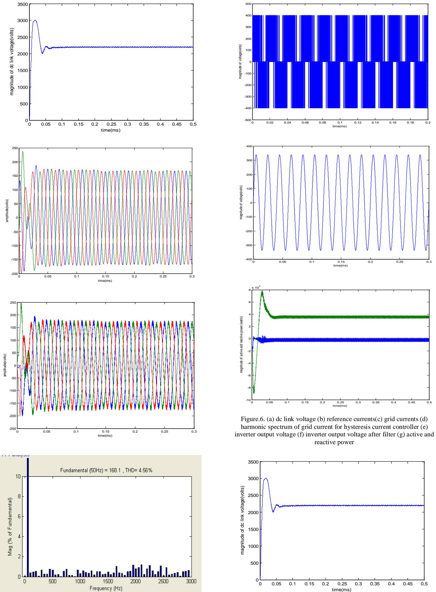
Figure.6. (a) dc link voltage (b) reference currents(c) grid currents (d) harmonic spectrum of grid current for hysteresis current controller (e) inverter output voltage (f) inverter output voltage after filter (g) active and reactive power
