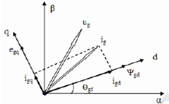
Figure 2 Virtual grid flux oriented reference frame
