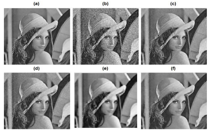
Figure 2. (a) Original image, (b) Noisy image( \sigma_n=30 ) (c) BayesShrink (d) Bilateral (e) ABF/Bayes (f) Proposed.
