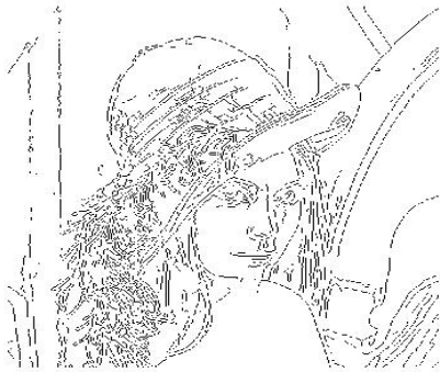
Figure 1. Edge detection using Canny method
