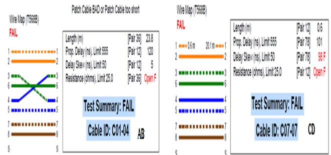
Figurers 4a: Test summary for Cable ID C01-04 (PATH: AB)      Figurers 4b: Test summary for Cable ID C07-07 (PATH: CD)
