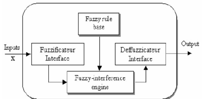
Figure 2. Basic Configuration of the fuzzy logic system
