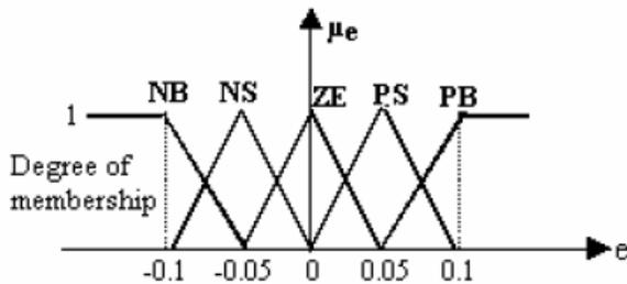
Figure 4. Membership Functions of Error
