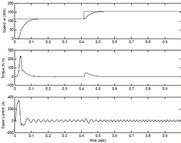
Figure 3. Speed Response Under no load torque
