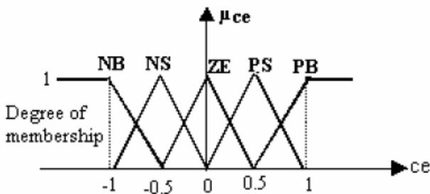
Figure 5. Membership functions of change in Error
