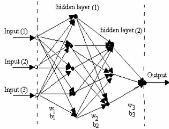
Figure 1. Architecture of Three Layer Neural Network
