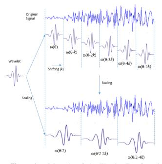
**Figure 1.** Schematic of the Wavelet Transformation Continues exemplifying two levels of resolution in 1D. Source: self-made.
