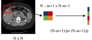
Fig 3. Example of convolution layer and pooling layer in two dimensions with an input of size N, one filter of size m and a pooling layer of size p.
