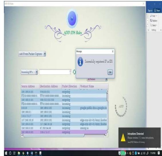
Fig 4: IDS rules is added and intrusion alert is shown as a desktop notification.
