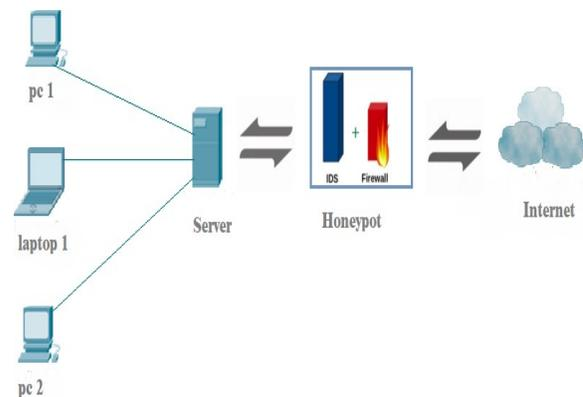
**Fig 1: The conceptual view of proposed frame work for Honeypot.**
