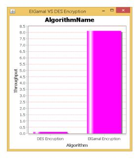
Fig 3. Elgamal and DES encryption Throughput
