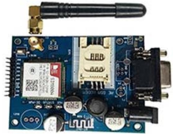
Figure 7. SIM800A GSM Board
