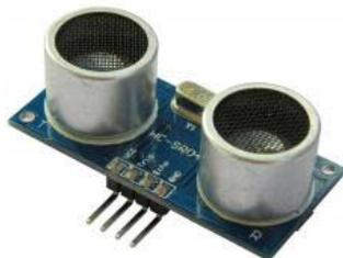
Figure 2. Ultrasonic sensor module: HC-SR04
