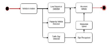
Figure 8. State Transition Diagram
