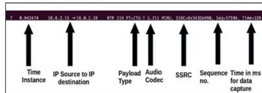
Figure 13. This figure illustrates the RTP data packet analysis
