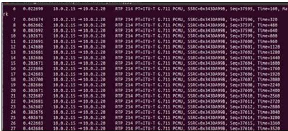
Figure 10. This figure shows the RTP packets of G.711 audio PCAP file
