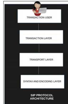
Figure 4. Illustration of an SIP Protocol architecture
