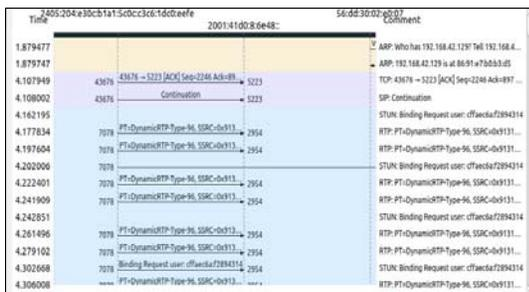
Figure 11. This figure shows the flowgraph of RTP packets of SIP.pcap file
