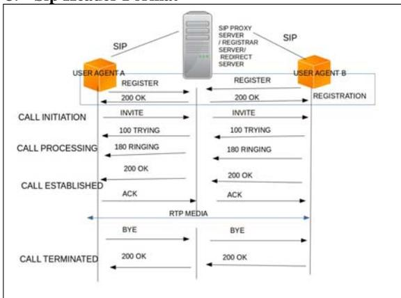
Figure 3. Illustration of an IP Phone call using SIP flow graph
