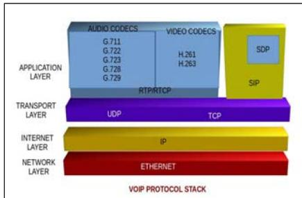
Figure 1. The protocol stack implementation of VoIP.
