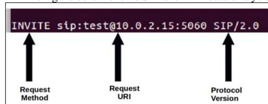
Figure 12. This figure illustrates the SIP data request header format
