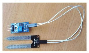
Figure 5. Capacitive Soil Moisture Sensor
