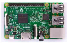
Figure 6. Raspberry Pi 3 Model B
