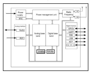
Figure 1. Sim800l Diagram (Simcom)[9]
