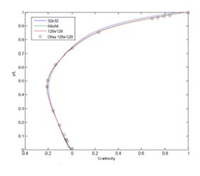
Fig. 3 U-velocity profile along the y-axis through the geometric center of the square cavity (Re = 100) with comparison to Ghia et al. [5].
