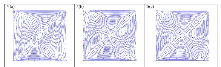
Fig. 5 Streamlines contours for different values of Reynolds number with horizontal walls are moving in opposite direction (a) Re=100 (b) Re=400 (c) Re=1000
