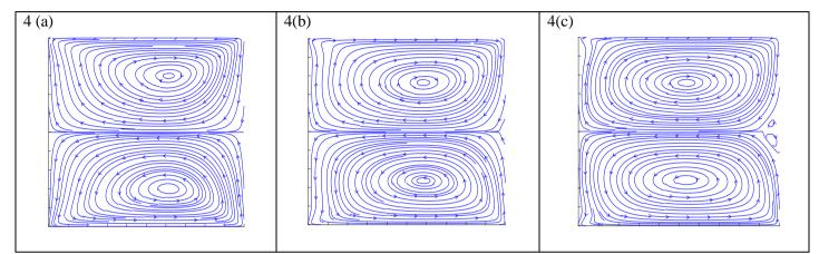
Fig. 4 Streamlines contours for different values of Reynolds number with horizontal walls are moving in same direction (a) Re=100 (b) Re=400 (c) Re= 1000
