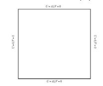
Fig. 1 Schematic diagram of the Square Cavity
