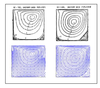
Fig. 2 Comparison of streamlines for our MAC method and results reported by Ghia et al. [5] for various Reynolds numbers
