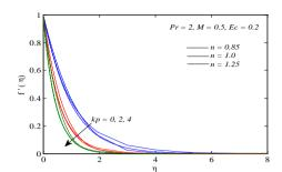
Fig.4 Velocity for different values of kp.
