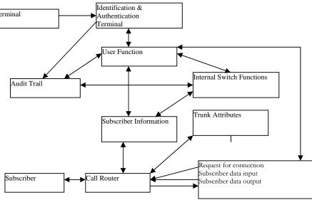
Figure 2: PBX Functional Architecture
