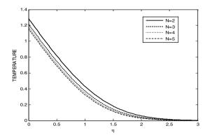
Fig.2. Effect of Radiation parameter N on temperature profiles with Pr=0.71, t=0.2
