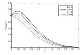
Fig.5 Effect of Grashof number Gr on velocity profiles with Gm=2, N=2, Sc=0.5, Pr=0.71, t=0.2
