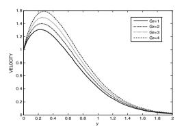
Fig.4. Effect of Grashof number Gr on velocity profiles with Gm=2, N=2, Sc=0.5, Pr=0.71, t=0.2
