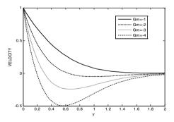
Fig.7. Effect of modified Grashof number Gm on velocity profiles with Gr=2, N=2, Sc=0.5, Pr=0.71, t=0.2
