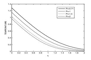
Fig.3. Effect of Prandtl number Pr on temperature profiles with N=2, t=0.2
