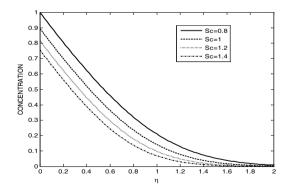
Fig.1. Effect of Schmidt number Sc on concentration profiles with N=2, t=0.2
