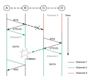
Fig.2.Multichannel hidden terminal problem. Channel is the control channel
