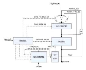
Figure.4: Modified block Diagram of Decryption Module
