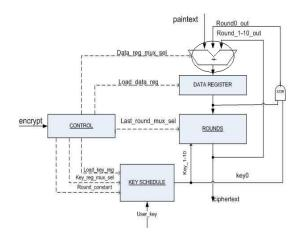
Figure.3: Modified block Diagram of Encryption Module
