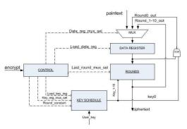
Figure.1: Basic block Diagram of Encryption Module
