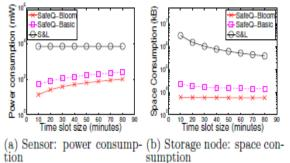
Figure 4: Ave. power and space consumption for 3dimensional data.
