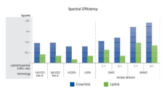
Figure 7. Mobile WiMAX vs. 3G Spectral Efficiency Comparison Source: WiMAX Forum [10].
