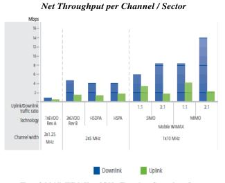
Figure 8. Mobile WiMAX vs. 3G Net Throughput Comparisons Source: WiMAX Forum [9].
