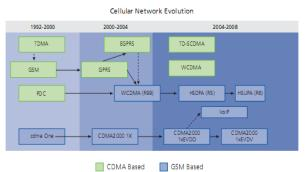
Figure 3. Cellular Network Evolution Source: Intel [2]
