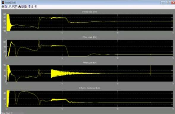
Fig. 7 Results Power input, Power main load, Power Secondary load.
