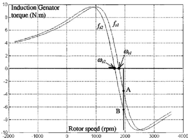
Fig. 2. Torque-speed characteristics of the induction generator, for different synchronous frequencies ( $f > f$ ).
