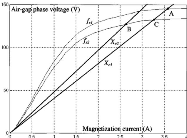
Fig. 3. Magnetization characteristics of the induction generator, for different synchronous frequencies ( $f > f$ ).
