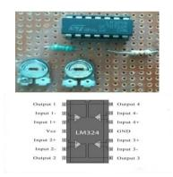
Figure 7: Comparator circuit
