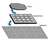
Figure 3: Photovoltaic panel or array
