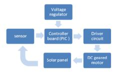
Figure 1: Block diagram of the project
