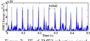
Figure 7: IE of IMF3 vibration signal of faulty gearbox
