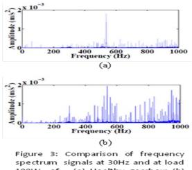
spectrum signals at 30Hz and at load 100W of (a) Healthy gearbox; (b) Faulty gearbox
