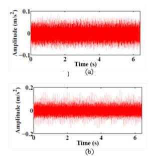
Figure 2: Comparison of time domain signals at 30 Hz and at load 100W of (a) Healthy gearbox; (b) Faulty gearbox
