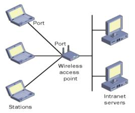
Figure 1. Wireless Components
