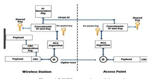
Figure 1.7 WEP encryption and decryption
