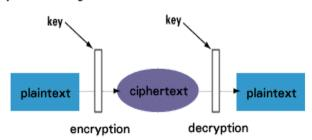
Fig 2: Symmetric key cryptographic algorithms process
