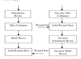
Fig 3: One Round of encryption and Decryption in AES
