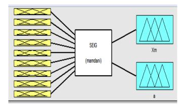
Fig.2. Fuzzy Model for SEIG to find Magnetizing Reactance and Generated Frequency
