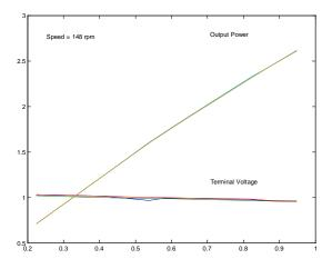
Effect of load admittance on terminal voltage and output power with air-gap voltage (E1= 1.00 pu)
