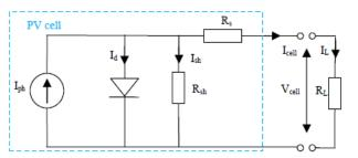
Figure 4. Equivalent Electrical circuit model of PV cells [37]
