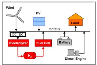
Fig 1. Block diagram of typical RES system[5]
