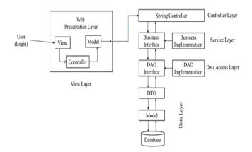
Figure 2. MVC Architecture layers of the proposed system.
