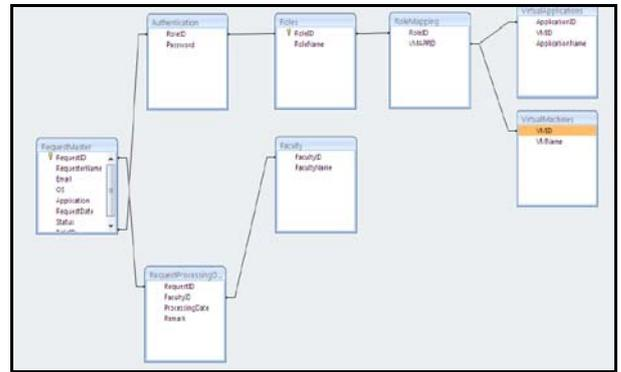
Figure 5. Database Structure for Front End Application
