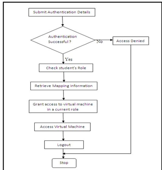
Control Flow Logic for Virtual Machine Access by Students
