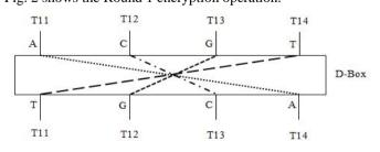
Figure 2. Round 1 Encryption Operation.
