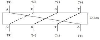
Figure 5. Round 4 Encryption Operation.
