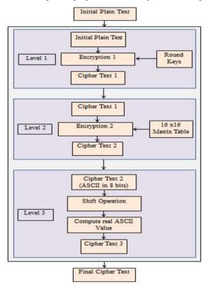
Figure 1. Block Diagram of Proposed Model [6].
