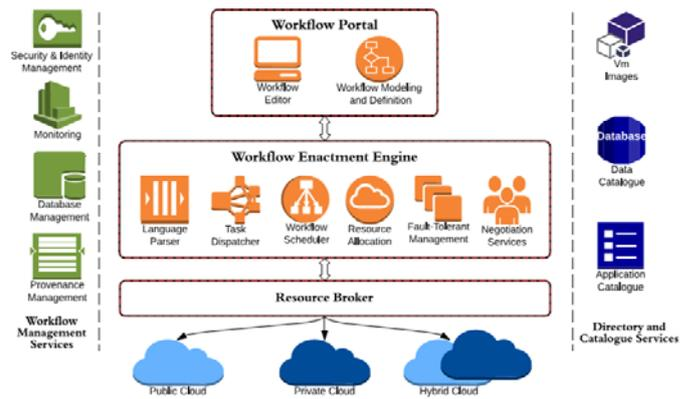
Figure 1.1: Architecture of cloud workflow management system.
