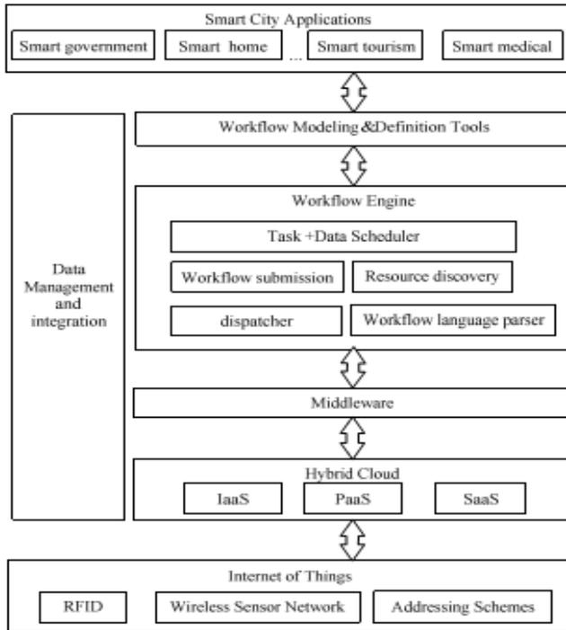
Figure 1.3. Cloud-based Workflow Architecture for Smart City
