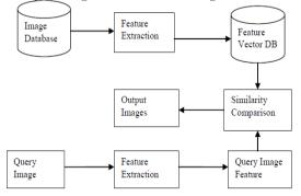
Fig 3: Block Diagram for CBIR Technique
