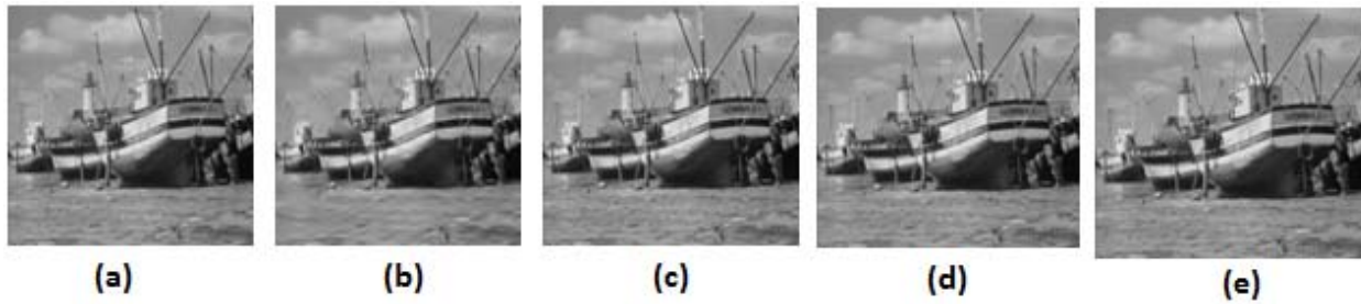
Fig. 4 (a) Original boat image compressed at compression ratio of 80:1 using (b) SPIHT (c)WDR;(d)JPEG2000[16];(e)Proposed method(Q=0.006)
