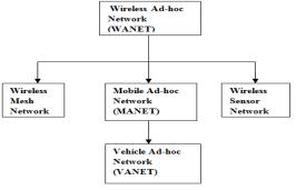
Fig 1: Hierarchy of Wireless Ad-hoc Network[6]
