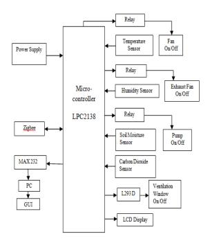
Fig.1.Block diagram of polyhouse automation
