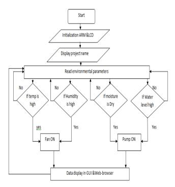
Fig 2: Flow chart of polyhouse automation
