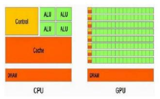
Fig2: Computational Resources of CPU and GPU [4]
