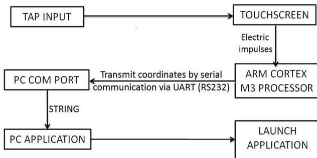
Figure 1. The system flow.
