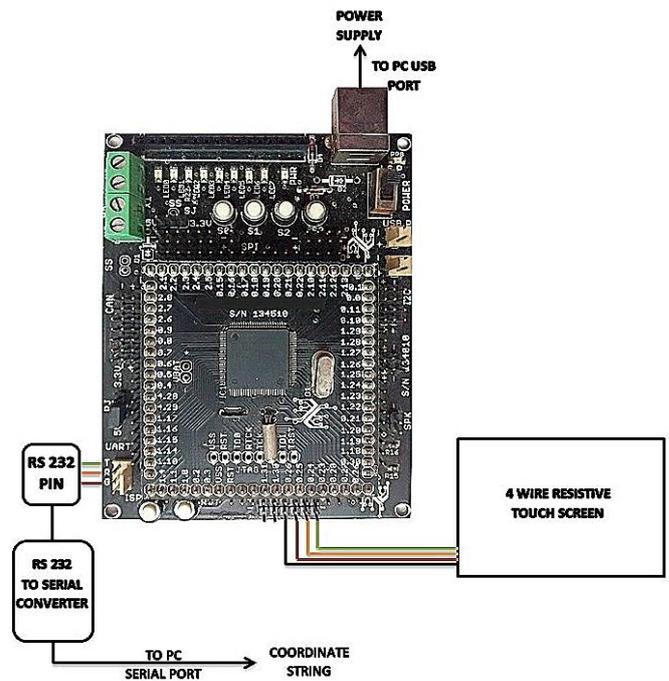
Figure 2. The hardware configuration.
