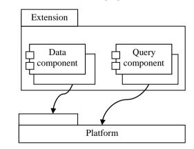
Figure 1: CMRS architecture comprises of a media independent platform and media specific extensions, which contain one or more *Data* and *Query* components
