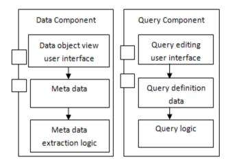
Figure 2: *Data* and *Query* components encapsulate the data, user interface and operations related to physical media items and queries, respectively.
