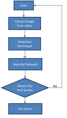
Figure 1.state diagram of detection of smoke
