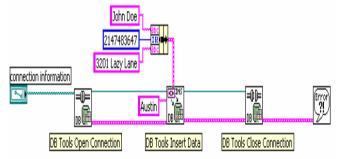
Fig 1: Basic Database Programming Model
