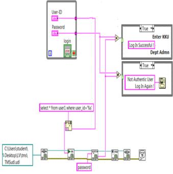
Fig 4: Block diagram of Login VI in LabVIEW for user authentication in KKU Dept Admn System
